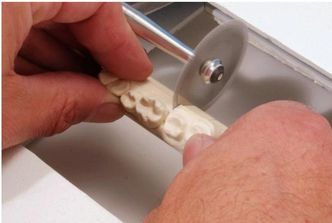
The blue table top can be flipped up to use the diamond disk lathe style for making buccal and lingual cuts or can be top cut with a hand saw to complete die section.
